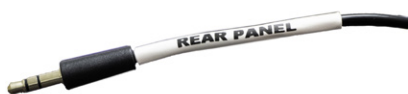
Fig. 7—The Foot Switch Connector is labeled “Rear Panel.” Do NOT plug it into the injection port on the front panel.
