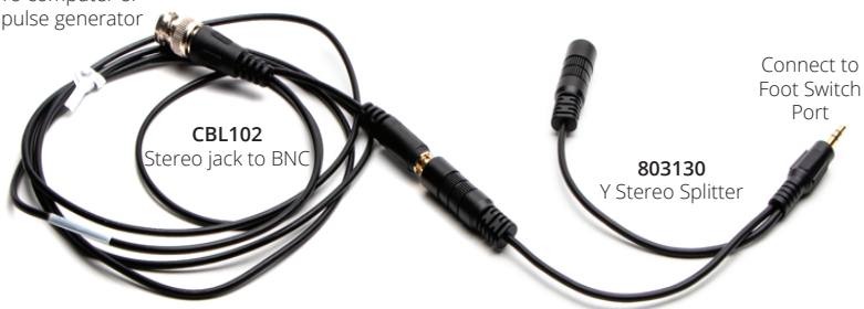
Fig. 14—Use the CBL102 and the 803130 to configure the system for a TTL trigger. The \mu Pump will inject on the high to low transition of the incoming TTL pulse.
